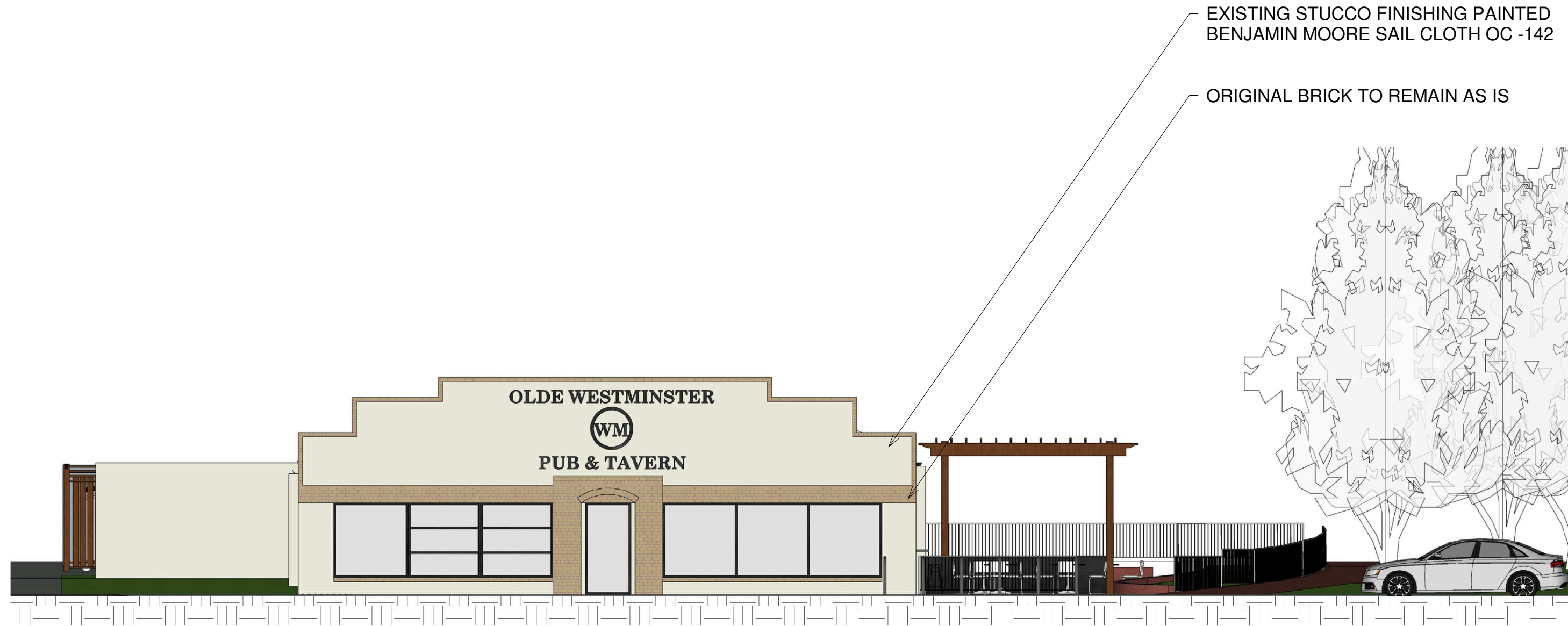
2 ODP - SOUTH ELEVATION 11 of 16 SCALE: 1/8" = 1'-0"
